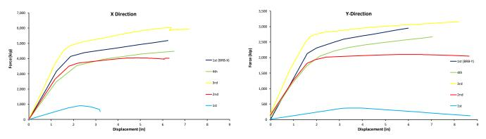
Figure 3. Non-linear storey backbone curves obtained from non-linear pushover analysis on each level, each orthogonal direction, including new BRBs on 1<sup>st</sup> level.
