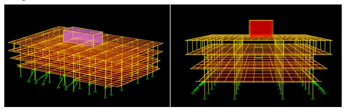
Figure 2. Views of the 3-dimensional model created in SAP2000, four storey steel moment frame portion of building.
