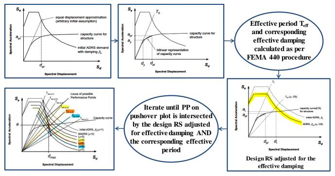
Figure 6. Equivalent linearization method of FEMA 440.
