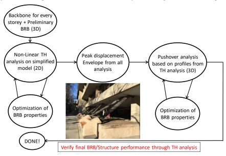
Figure 8. Analyses flowchart in the design and optimization.
