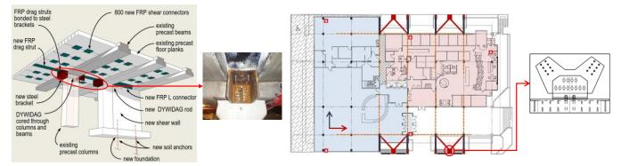
Figure 9. FRP drag strut to steel bracket connection to provide continuity of load path through columns and into the shear walls(left side of figure); layout of drag struts (red dotted lines) relative to BRBs and slotted connection at base of V-configured BRBs.
