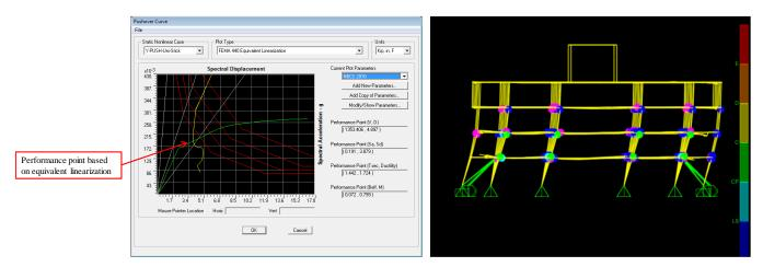
Figure 7. Equivalent linearization method in SAP2000 and hinge formation throughout the structure at the performance point.
