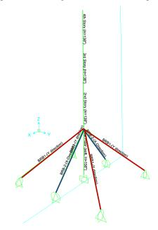
Figure 4. Simplified stick model of the structure for use in non-linear time-history analysis.
